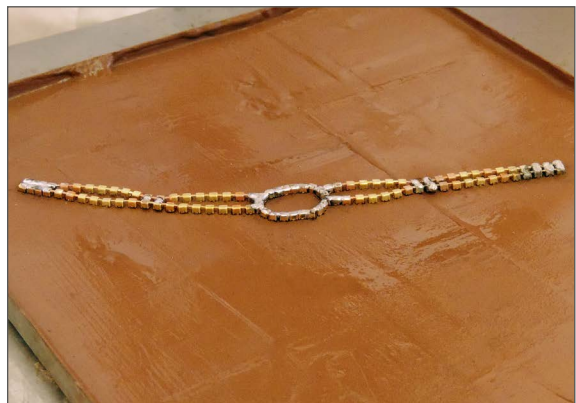
12 After soldering, let the product cool down.
