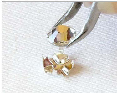
Setting the stone into the cup
