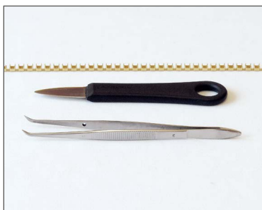
Tools for closing the cup by hand
