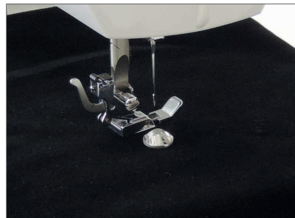
Application of crystals with the lower feed switched off.
